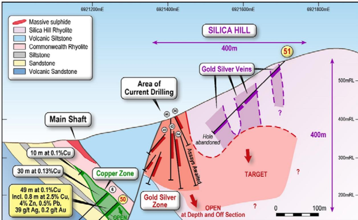
**Figure 3.** Cross section looking northwest from Main Shaft to Silica Hill. Three components to the mineralised system are evident: an upper zone of weakly mineralised gold-silver veins; a middle zone of high grade gold-silver +/- base metal veins; and a lower zone of massive sulphide and increasing copper-gold-silver at depth.
