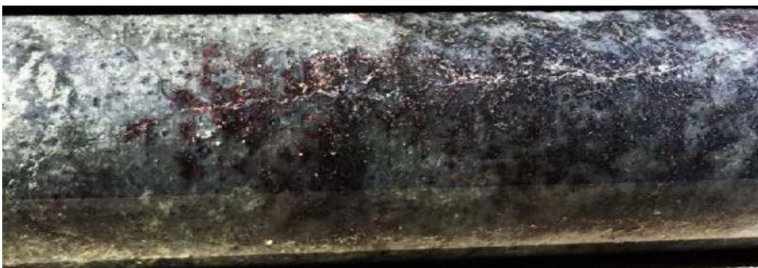
**Figure 5.** Quartz-pyrite-arsenopyrite-silver vein and stockwork from 77 m depth in Hole 63.
