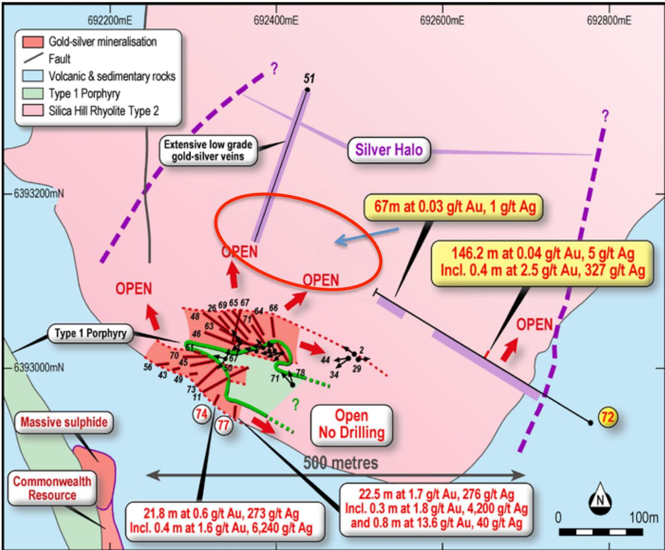
**Figure 8.** Silica Hill Prospect: Geology, drill hole locations and recent significant results. The mineralisation is open and large areas remain to be drill tested.
