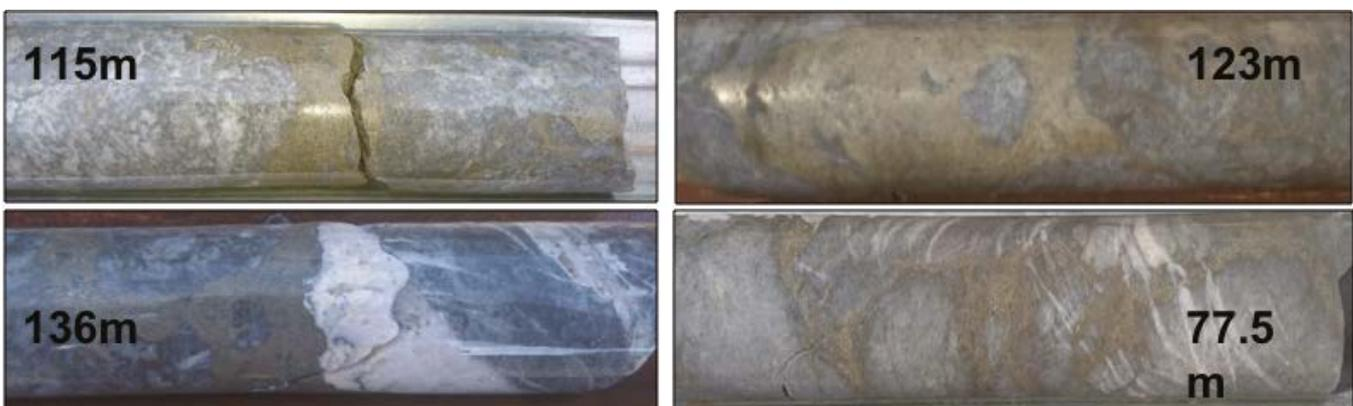
**Figure 7.** Examples of pyrite-arsenopyrite vein styles and orientations from Hole CMIPT64 from down hole depths shown. Similar veins are seen in Holes 65 and 66. All contain silver.
