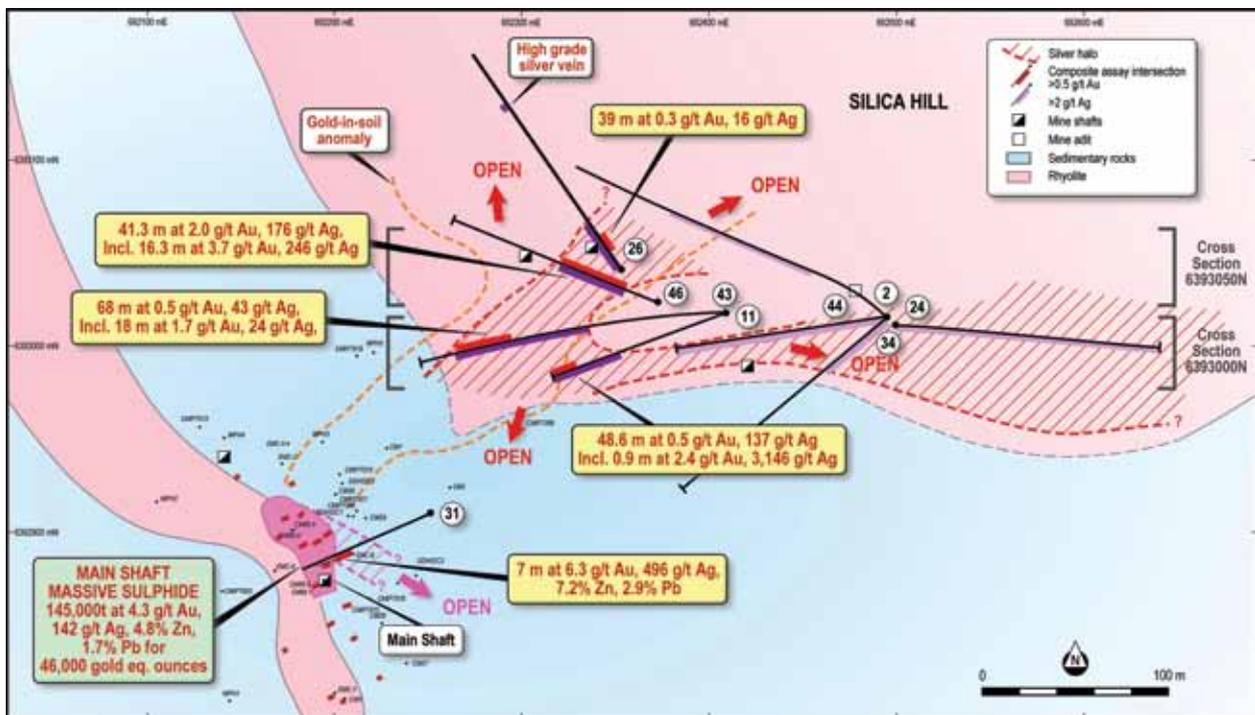
**Figure 4.** Surface geology map showing significant drill intercepts at Silica Hill and Main Shaft.
