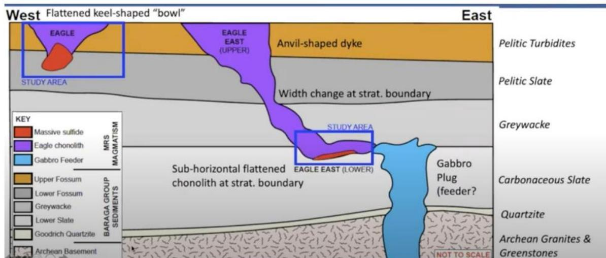
**Figure 5:** Simplified cross-section through the Eagle and Eagle East deposits.
