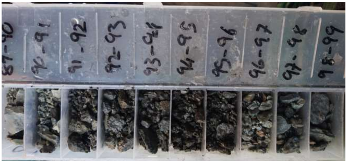
Figure 3. RC drill chips from CMIPT031 showing massive sulphide from 91 to 98 m.
