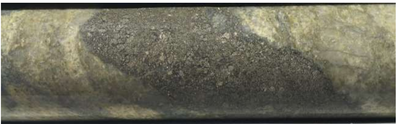
Figure 7. High grade silver-pyrite vein from CMIPT026. The vein contains up to 400 g/t silver as measured with the handheld XRF instrument.
