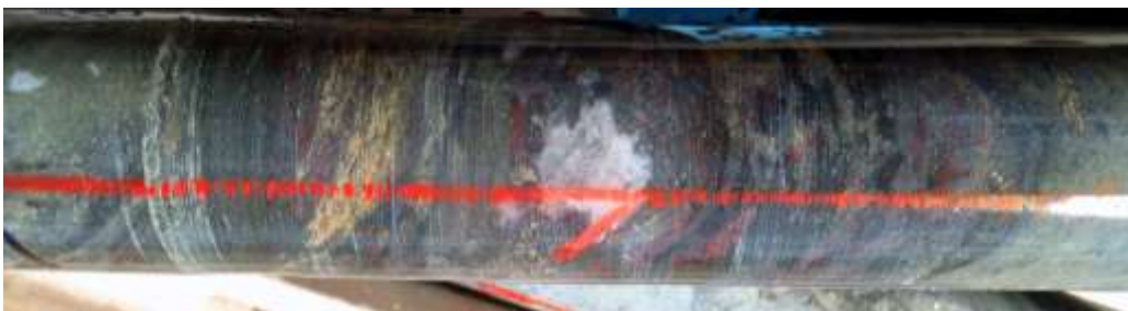
Figure 1. Veins of visible silver minerals (red-purple colour) from Hole CMIPT077 from 174.4 m which assayed 1.8 g/t gold and 4,200 g/t silver over 0.3 metres
