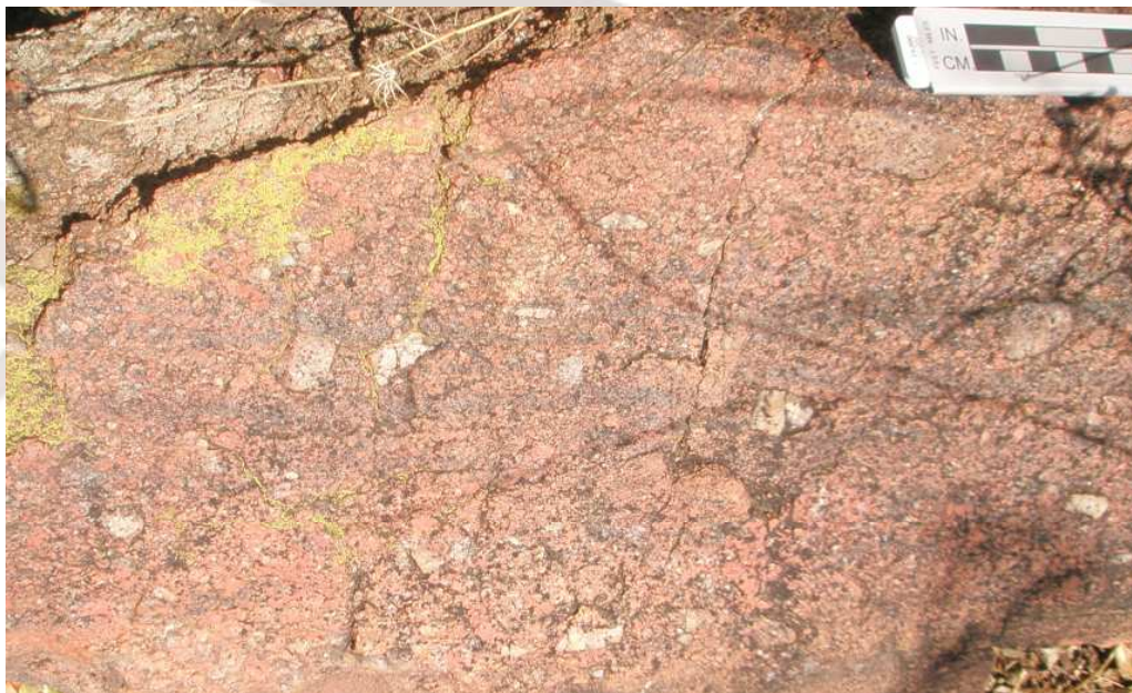
Figure 3a. Haematite-chlorite altered conglomerates of the Palapye Group from the Kodibeleng area with uranium values of up to 100 ppm eU 3 O 8 .
