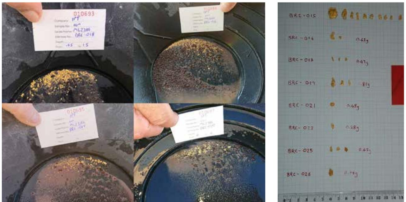
**Figure 25:** Examples of the panned concentrates from Foxes Lead on ML2386 and picture of nuggets from all trenches. All gold is the property of Impact Minerals Limited.
