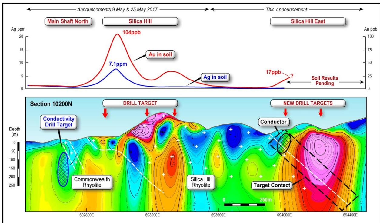
**Figure 6.** Section Line 10,200 mN (Figure 7) showing IP chargeability data from Main Shaft North to Silica Hill East. Note the size and strength of the Silica Hill East anomaly and increasing gold-in-soil response over the target contact and associated conductor.
