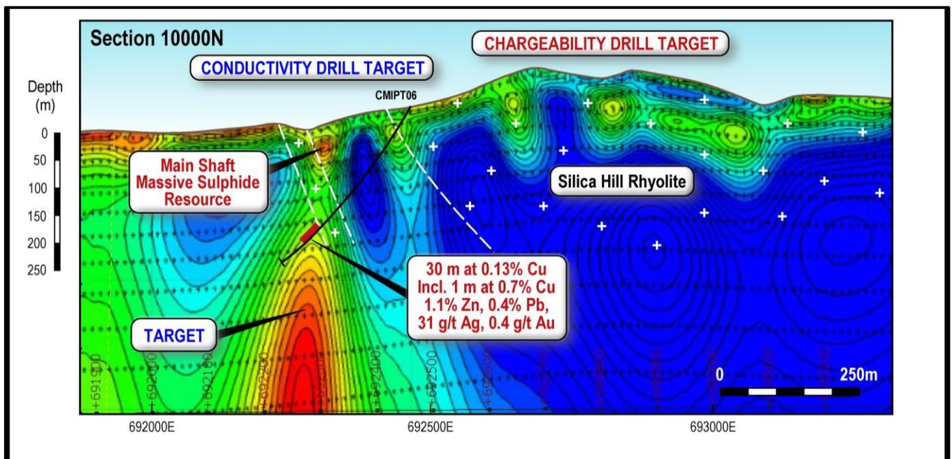
**Figure 3.** IP Conductivity data along Section 10,000 mN showing the massive sulphide body at Main Shaft and copper-rich drill hole CMIPT06.
