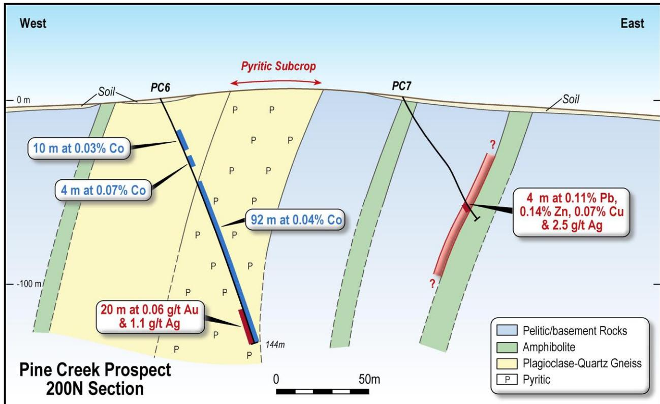
Figure 15. Geology and significant drill results of the Pine Creek Project. Note the mineralisation is open at depth.
