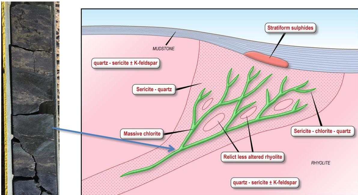
**Figure 11.** Conceptual model of feeder zone and related massive sulphide from published scientific papers on Eskay Creek. Also shown is drill core and the interpreted position of a “feeder vein” at Silica Hill with strong chlorite (dark green) alteration in the high grade sulphide intercept in CMIPT011 of **0.9 metres at 2.4 g/t gold and 3,146 g/t silver**.
