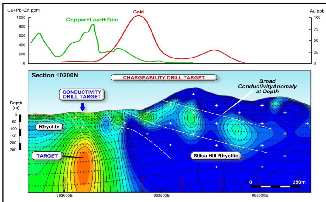
**Figure 4.** IP Conductivity data along Section 10,200 mN showing coincident IP conductivity and lead-zinc-copper-in-soil anomalies. The gold-in-soil anomaly is coincident with strong IP chargeability anomalies (see announcement [9 May 2017](#)).
