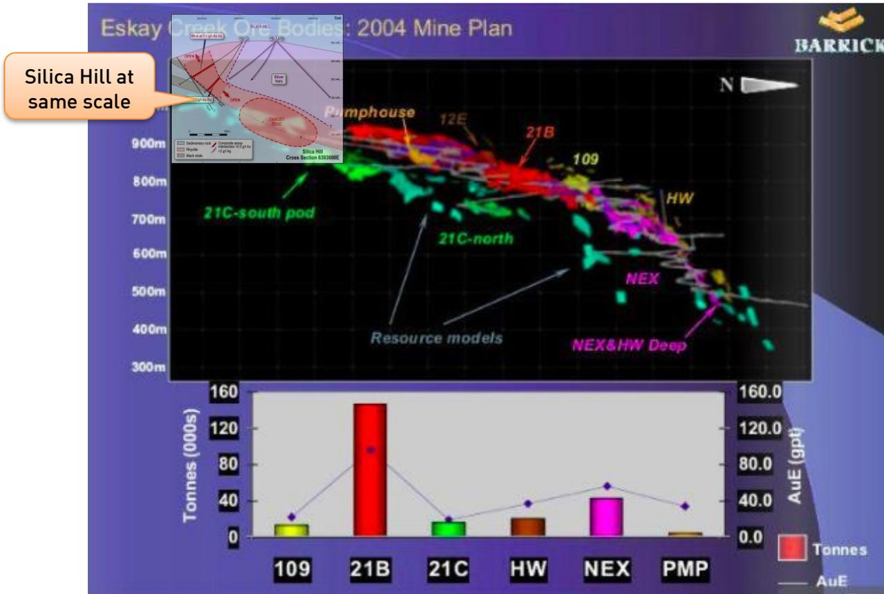
**Figure 10.** Long section of the Eskay Creek gold mine showing the principal ore shoots (eg 21B, NEX etc) coloured by gold equivalent grade. The graph shows the tonnes and gold equivalent grade of each of the shoots. Also shown for comparison at the same scale in the top left hand corner is the cross section of Silica Hill (image is slightly transparent in order to show the upper most Eskay Creek ore shoots).
