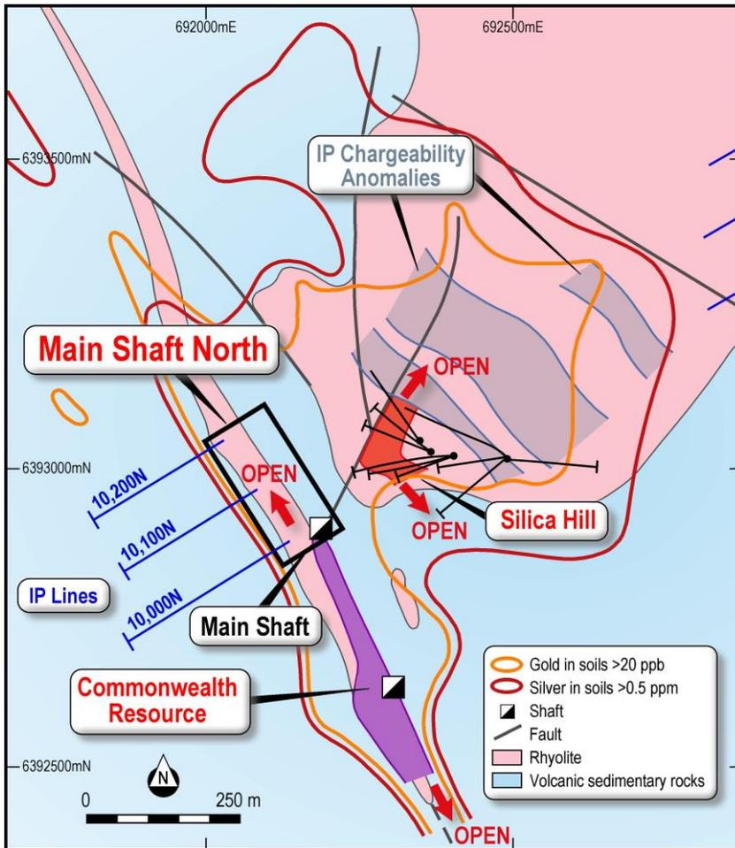
**Figure 1.** Geology and exploration results for the Silica Hill-Commonwealth-Main Shaft area. The Silica Hill mineralisation, shown in red, lies 150 metres north east of the Commonwealth Resource and occurs at the southern end of a large area with coincident gold- and silver-in soil and IP chargeability anomalies that has not been drilled.
