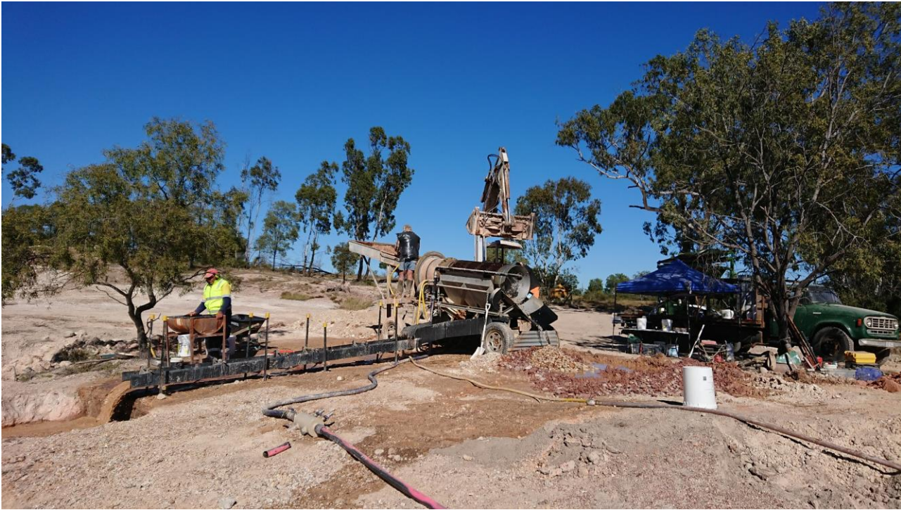
Figure 3. Impact's water processing set up for the bulk samples at Black Ridge.
