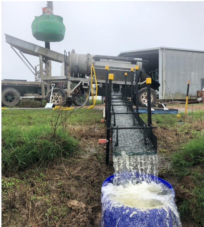
Figure 2. Commissioning of Mobile Wet Processing Plant for Gold
