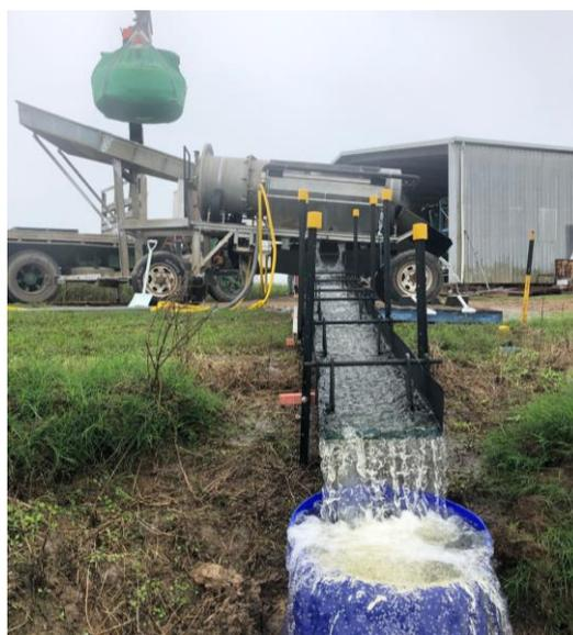
**Figure 1.** Commissioning of Mobile Wet Processing Plant for Gold
