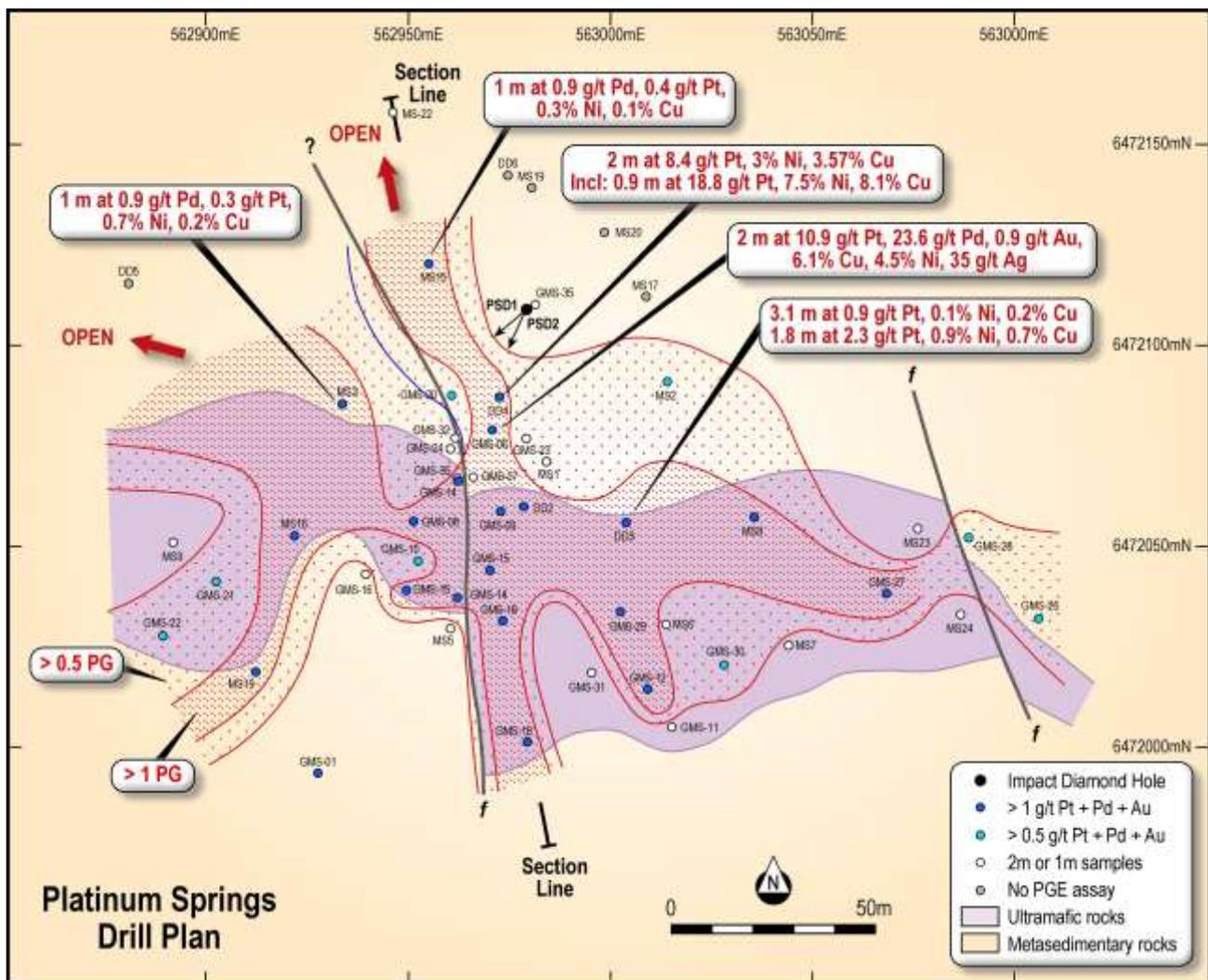
**Figure 1.** Geology and location of PSD01 and PSD02, previous drill holes and contoured data of previous drill assays for platinum, palladium and gold (summed from down hole intervals).
