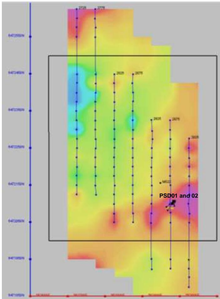
**Figure 2.** Image of late time EM data over the Platinum Springs Prospect showing the location of Impact drill holes PSD01 and PSD02.
