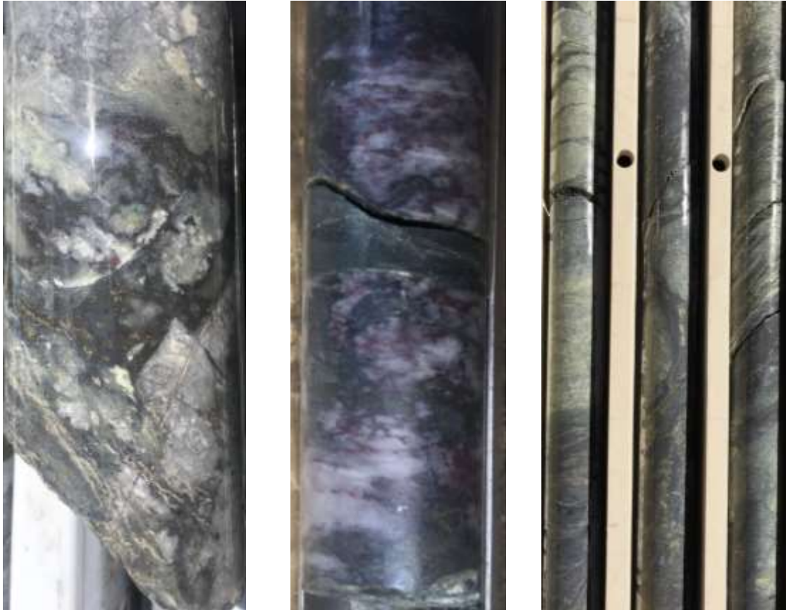
Figure 3. Veins of visible silver minerals (red-purple colour) from Hole 072 (left) and Hole 073 (middle) and massive sulphide veins (dark colour) also from Hole 073.
