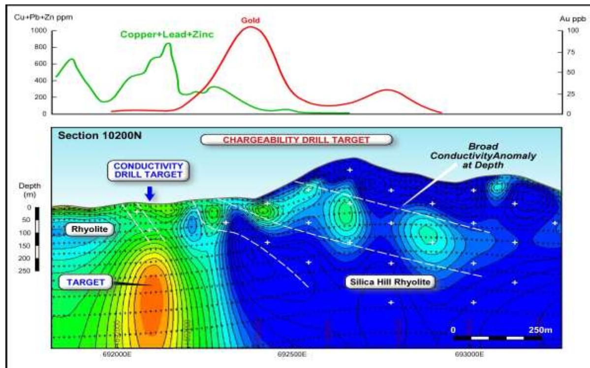
**Figure 3.** IP Conductivity data along Section 10,200 mN showing coincident IP conductivity and lead-zinc-copper-in-soil anomalies. The gold-in-soil anomaly is coincident with strong IP chargeability anomalies (see announcement [9 May 2017](#)).
